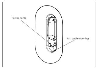
Push power cable through rubber plug. Place lamp base flush to the mounting surface.
