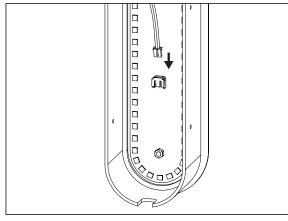
Connect the plug from the driver to the connector on the LEDmodule.
