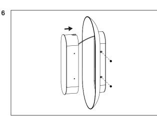
Attach the diffuser and LEDmodule to the lamp by placing it into the shade and tightening the 4 screws on the sides of the lamp.
