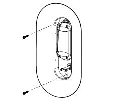
Mount the lamp to the wall or ceiling with screws.
